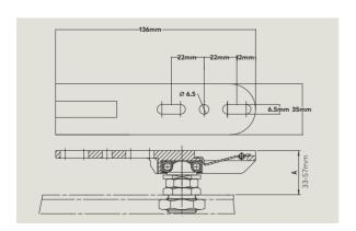
RTS Pivot Set End Load Threshold Mounted (85210023)
